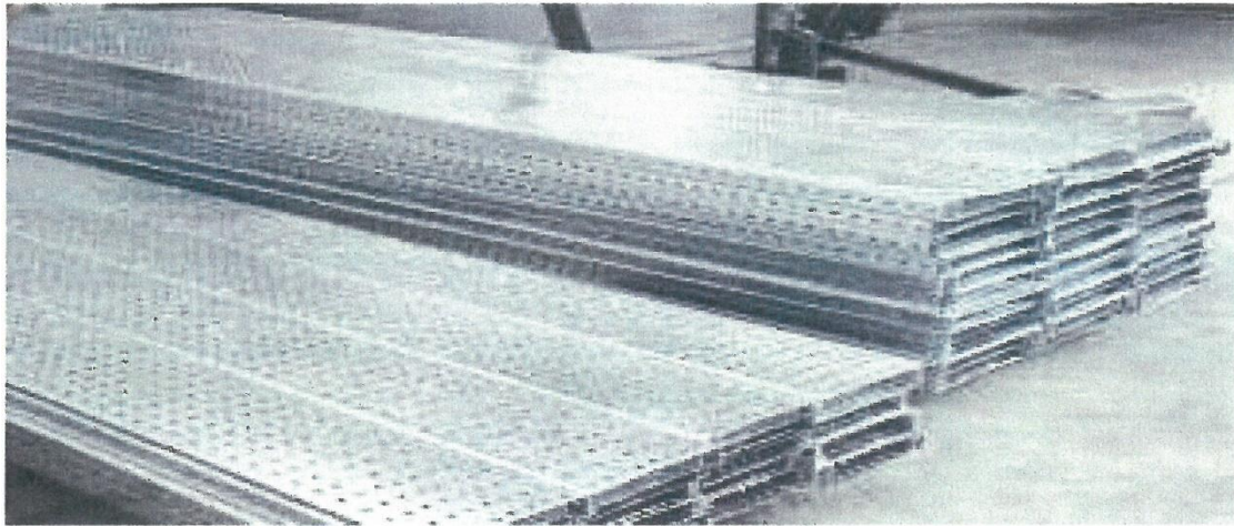
(Figure-3) Sample Picture (Cable Tray Storage)
