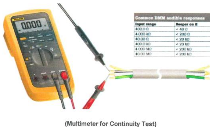
Figure-7 (Sample Picture) – Multimeter for Continuity Test
