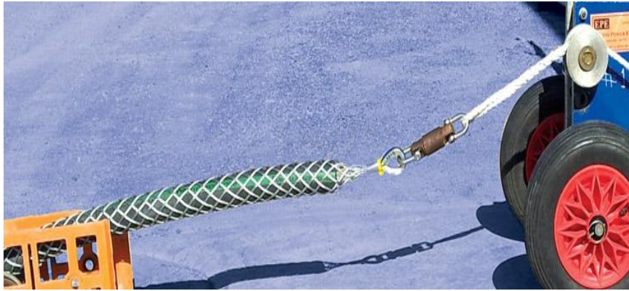
Figure – 14 (Sample Pic) Cable Sock and Winch Machine for Cable Pulling
