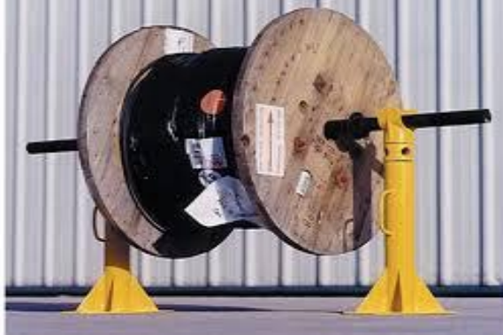
Figure – 12 (Sample Pic) Cable Drum installed on Jacks with Spindle
