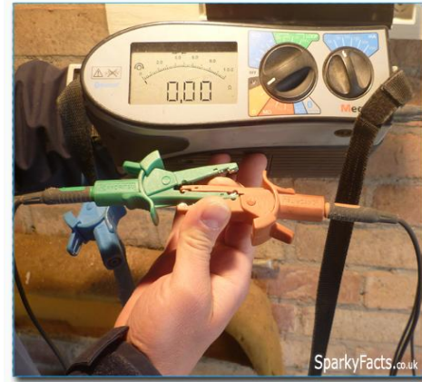
Sample Figure - 12 (Configuring Test Equipment For Null)
