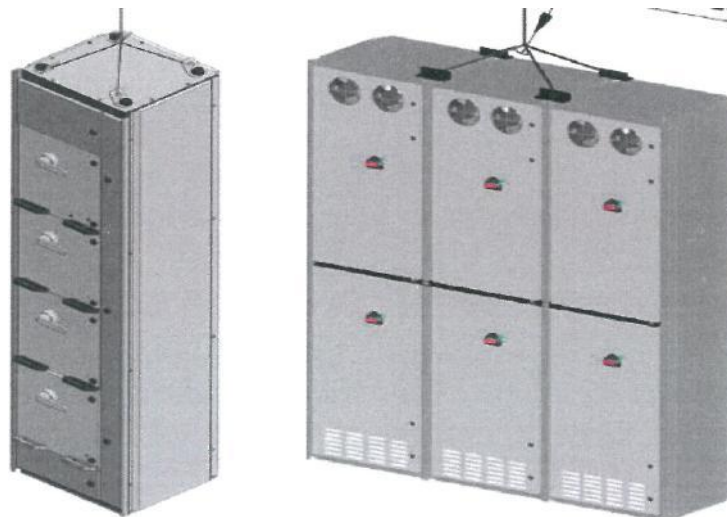
Sample figure 2: Overhead lifting industrial control panel with lifting angle
