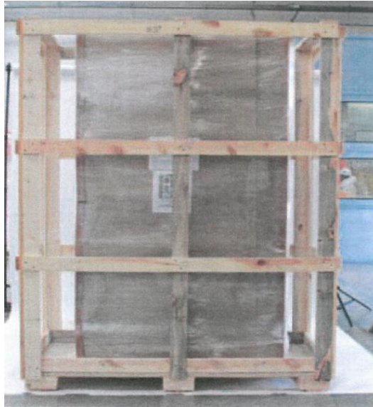
Sample figure 3: Storage of MCC Panel
